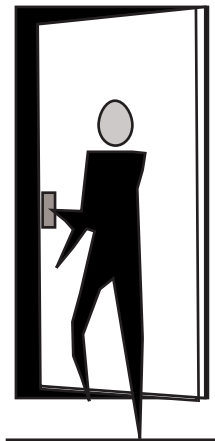
Right hand: hinges on right, opens inward
