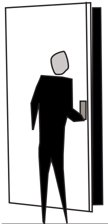
Left hand reverse: hinges on left, opens outward
