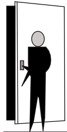
Right hand reverse: hinges on right, opens outward
